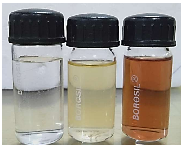
Fig. 1: Visual observation of Synthesis of silver nanoparticles (A) AgNO 3 solution, (B) Bacterial extract, (C) synthesized silver nanoparticles
