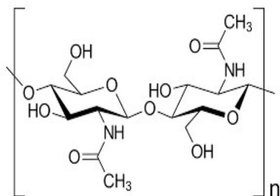
Fig. 1: Chemical structure of chitin
