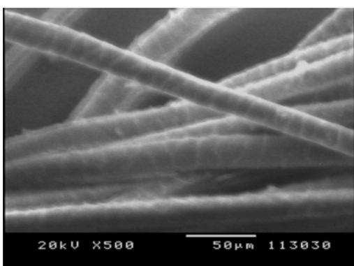
**Plate 2: acid treated fibers**
