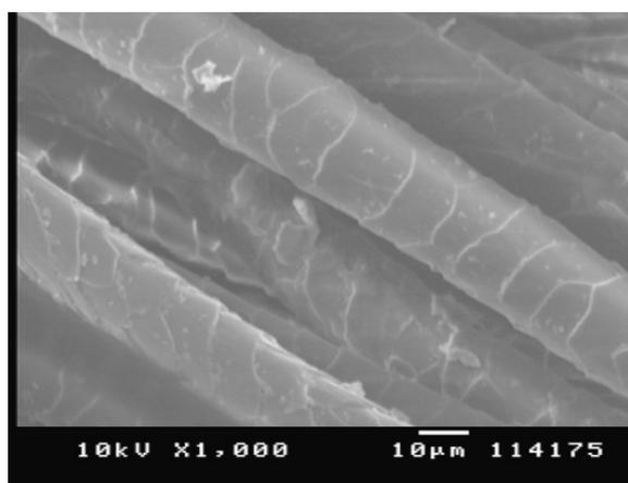
**Plate 4: Acid Enzymes Treated Sample With 10% Microwave Dyeing**
