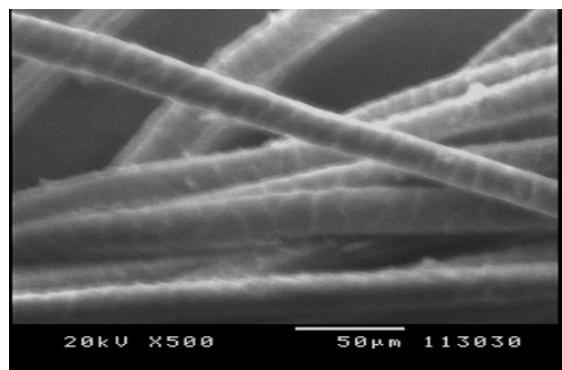
**Plate 3: Alkaline treated fibers**
